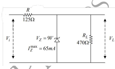
(A)  $V_i^{min} = 9.0$  V and  $V_i^{max} = 11.4$  V
