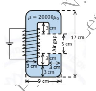
Ignoring the fringe fields, the magnitude of the magnetic field  $\vec{B}$  (in Tesla, rounded off to two decimal places) in the air-gap between the magnetic poles is
