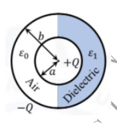
The electric field at a radial distance r from the center and between the shells (a < r < b) is
