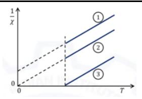
(Curie temperature of ferromagnetic material =  $T_C$ Néel temperature of antiferromagnetic material =  $T_N$ )
