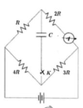
key K is closed, the reading in the ammeter is 27 mA. What will the reading (in mA) be a long time later?
