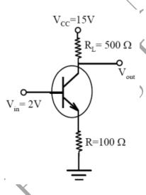
Assuming that there will be a 0.7 V drop across a forward-biased silicon p-n junction, the power dissipated across the transistor will be, approximately,
