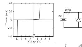
When this diode is used in the circuit on the extreme right, the approximate current, in mA, through the diode will be
