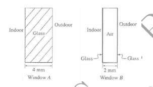
Window A is a simple pane of glass, A mm thick Window B, on the other hand, consists of two extremely thin panes of glass, separated by an air gap of 2 mm, as shown in the figure above. If the thermal conductivity of glass is known to be 0.8 Wm<sup>-1</sup>K<sup>-1</sup> and that of air is  $0.025 \text{ Wm}^{-1}\text{K}^{-1}$ , then the ratio of heat flow  $Q_A$  through Window A to the heat flow  $Q_B$  through Window B is given by  $\frac{Q_A}{Q_B}$
