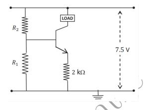
What will be the ratio of the resistances  $R_2/R_1$ , in order to make this circuit function as a source of constant current, I = 1 mA?
