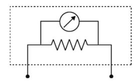
Such a realistic voltmeter, with input resistance  $1 k\Omega$ , gives a reading of 100 mV when connected to a voltage source with source resistance 50  $\Omega$ . What will a similar voltmeter, with input resistance 1 M $\Omega$ , read in mV, when connected to the same voltage source?
