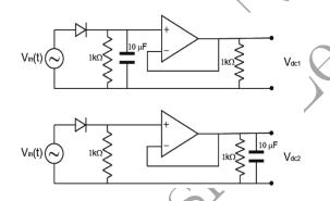
If the DC output voltage of the top circuit has a value  $V_{\rm dc1}$  and the bottom circuit has a value  $V_{\rm dc2}$ , then which of the following statements about the relative value of  $V_{\rm dc1}$  and  $V_{\rm dc2}$  is correct?
