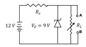
If a Zener diode with ratings,  $V_Z = 9$  V and  $P_{\text{max}} = 0.27$  W, is connected as shown in the figure, for the above purpose, the minimum series resistance  $R_S$  must be
